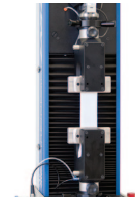
Pneumatic Clamps for medium-heavy fabrics, up to 300 Kg capacity approx., Code 2512E.730
