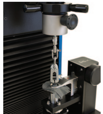
Upper Stud Grip ( Code 194E.12 ), Lower Fabric Clamp ( Code 194E.4 ), to test male parts of baby snaps, etc.
