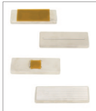
Example of interchangeable jaws, rubber/knurled, Grab, Contact Line, etc.
