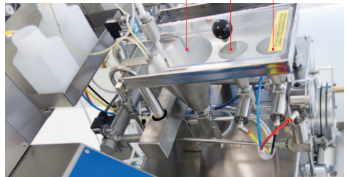
Picture showing the 3 automatic dosing tanks.
