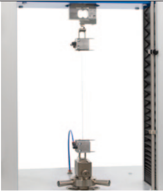
Pneumatic clamps for delicate yarns (POY, Lycra, cotton, worsted yarns), 20N max capacity, Code 2510.978
