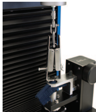
Upper ( Code 194E.16 ) & Lower ( Code 194E.14 ), Grasp Button Kit, & Lower Fabric Clamp ( Code 194E.4 ), for buttons, etc.
