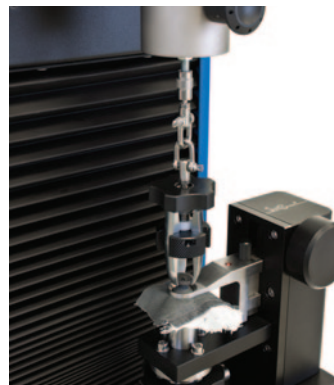
Upper Universal Grip ( Code 194E.6 ), Lower Fabric Clamp ( Code 194E.4 ), for buttons, etc.
