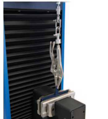
Upper Long Nose Vise Grip, for trousers' hooks and other accessories, according to M&S P115 (for buttons), Code 194E.10
