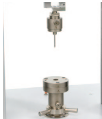
Perforation Testing Kit according to EN 388 Standard, Code 2510.681
