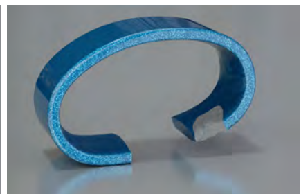
Incorrect Wear Pattern Different Style Required
