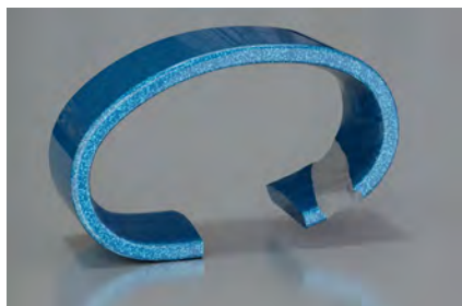
Excessive Wear Pattern Traveler Should Be Changed
