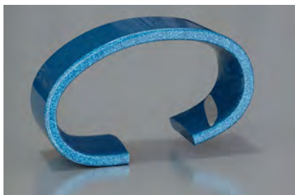
Normal Wear Pattern Proper Working Conditions
