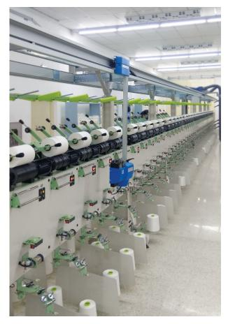
The Air Track Supply (ATS) system shown here contains the air hose inside the track. Track mounting location depends on machine configuration. Tracks can be mounted at the top or bottom of the machine, and different splicers can be used.
