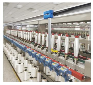
The **Air Track Supply (ATS)** system shown here contains the air hose inside the track. Track mounting location depends on machine configuration. Tracks can be mounted at the top or bottom of the machine, and different splicers can be used.
