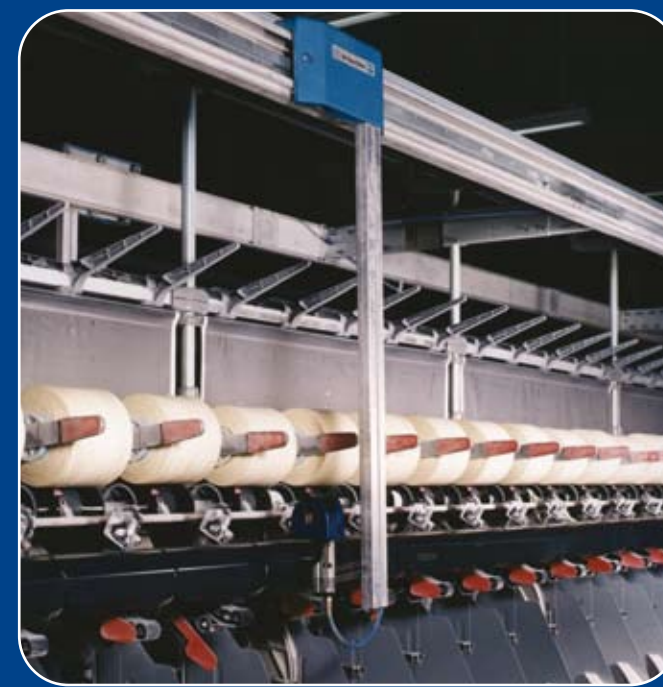
ATS "C" type with Jointair 115 installed on two-for-one twister.
