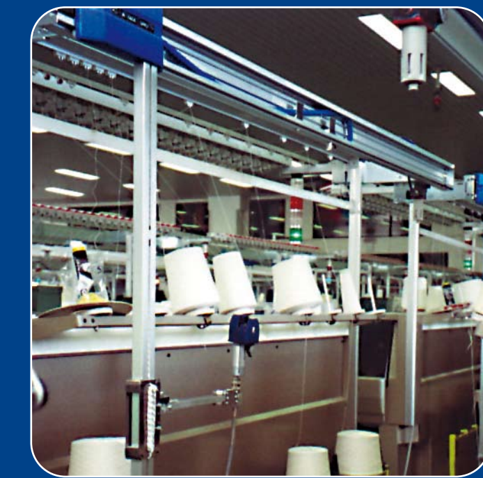
ATS "C" type with Jointair 115 on flat knitting machine.
