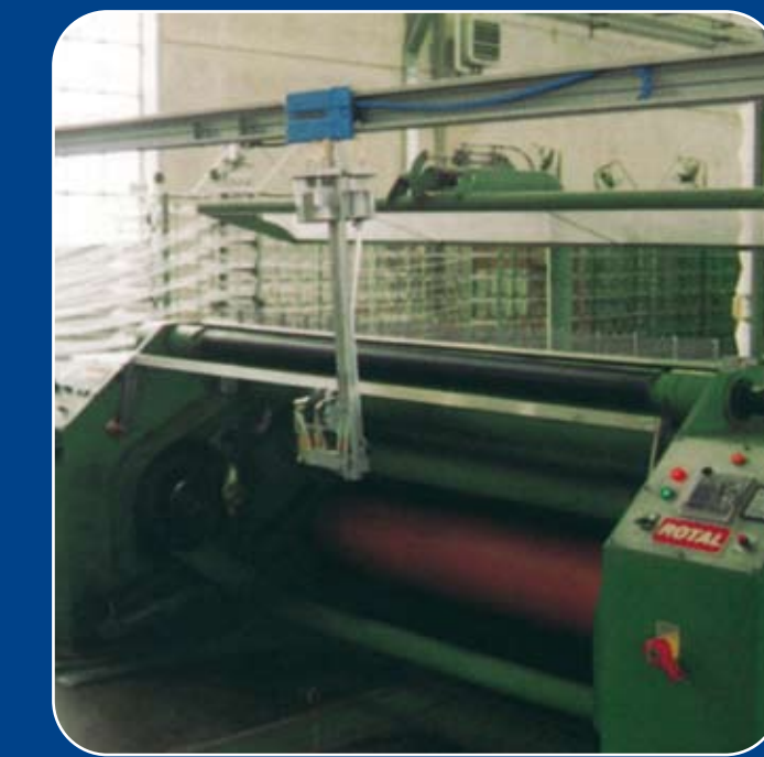
ATS "L" type with Aquasplicer 928B placed in front of a fractional warping machine for cotton yarn.
