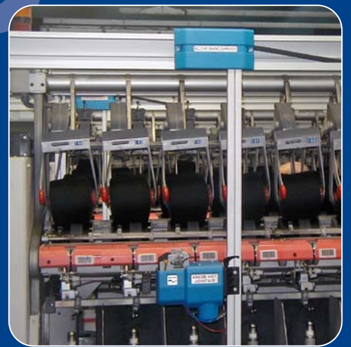
ATS "H" type with Hot Jointair 4983B installed on a two-for-one twister processing worsted yarn.
