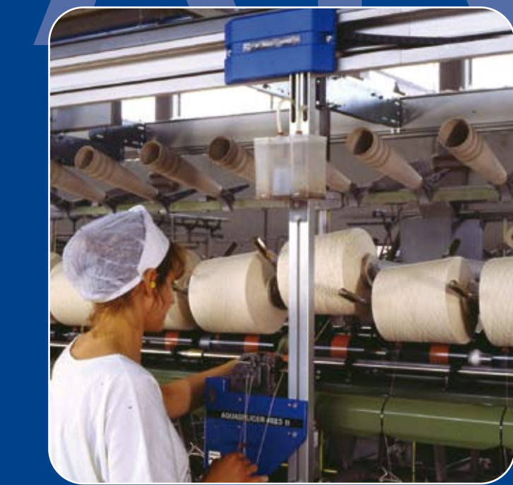
ATS "L" type carrying Aquasplicer 4923B in the most common installation from above on a two-for-one twister processing cotton yarn.
