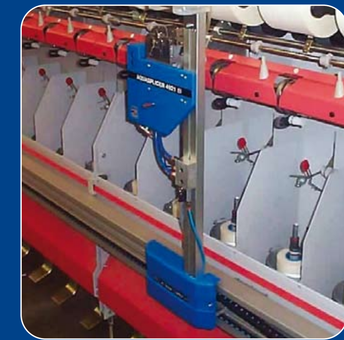
ATS "L" type with Aquasplicer 4923B installed from below on a two-for-one twister processing cotton yarn.
